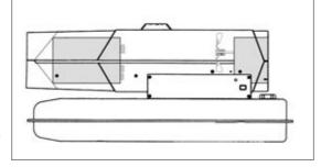
front of the fuel intake it causes fuel to rise from the tank and into the burner nozzle. This fuel and air mixture is then sprayed into the combustion chamber in a fine mist.
